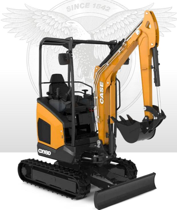
Engine 3TNV70 Engine power 11.3 kW - 15.4 HP Operating weight with canopy 1830 kg Operating weight with cab 1940 kg
