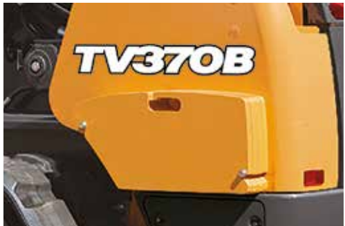
Additional Counterweight to increase ROC
