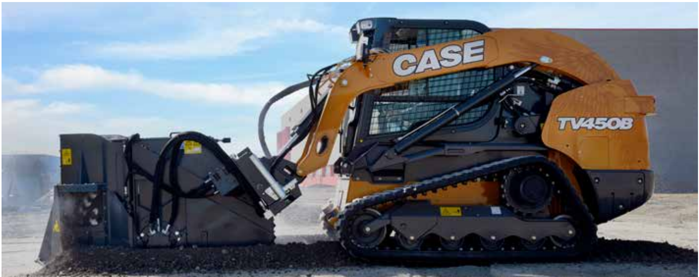
Additional Counterweight to increase ROC
